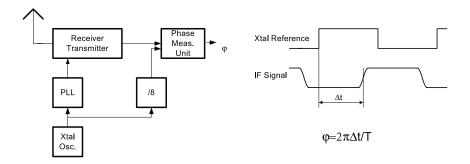
Atmels Active Reflector method overcomes synchronization
