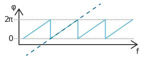
Distance *d* is proportional to slope  $m = \frac{\Delta \varphi}{\Delta f}$
