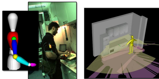
Fig. 5. Food preparing experiments in the AwareKitchen together with the 3d reconstruction of the person's motion from XSens IMUs (left) and a visualization of the person's position from the 3 laser sensors, during another experiment in the AwareKitchen (right).
