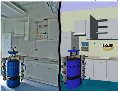
Fig. 3. Virtual and physical kitchen: the real environment is modeled and its physical properties are described so that sensors can acquire e.g. position, orientation, material density or gravity.
