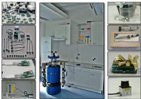
Fig. 4. The AwareKitchen is an example for a sensor augmented intelligent environment. Everyday objects are tagged with RFID markers and partially equipped with wireless sensor nodes. Off-the-shelf and custom made components turn objects into context providers. Magnetic sensors in all doors detect opening and closing events. Mica2, Motes, Particles and Porcupine wireless sensor nodes enable unobtrusive data acquisition. RFID readers in the kitchen shelves detect the addition and removal of objects in various places, e.g. cupboards, tables, etc. An intelligent cutting board and a sensor knife enable context acquisition in the course of food processing and meal preparation. Laser scanners provide the position and number of people working in the kitchen. Robots learn from human behavior, e.g. from movement trajectories captured by inertial sensors and help completing tasks as part of the assistive health-care technology.
