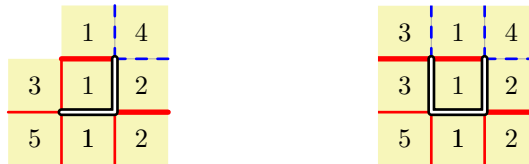
Figure 15: Crease pattern around an L-slit (left) and a U-slit (right). Numbers indicate the face of the six-sided die in the folded state; thinner lines denote creases folded by \pm 90^\circ ; thicker lines denote creases folded by \pm 180^\circ ; mountain folds are drawn solid/red; and valley folds are drawn dashed/blue.
