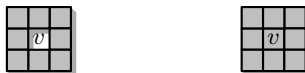
■ Figure 4 Meta-modules are either clean or solid, depending on whether the center cell is occupied.
