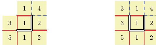
Fig. 15. Crease pattern around an L-slit (left) and a U-slit (right). Numbers indicate the face of the six-sided die in the folded state; thinner lines denote creases folded by \pm 90^\circ ; thicker lines denote creases folded by \pm 180^\circ ; mountain folds are drawn solid/red; and valley folds are drawn dashed/blue.
