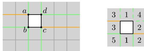
Figure 9: Left: crease pattern around a hole folding into an L-shape when gluing vertices a and c ; 90^\circ creases are shown in green, and 180^\circ creases in orange. Right: numbers indicate the face of the cube in the folded state; mountain folds are shown in solid, and valley folds as dashed lines.
