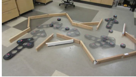
Fig. 2 A potential application of object characterization in collective transport: by computing the centroid and orientation of the object, a swarm of manipulator robots can maneuver the object to valid free configurations and safely transport the object
