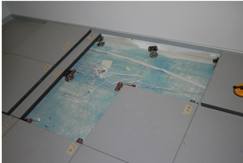
(b) Load sensors attached to iSense node.
