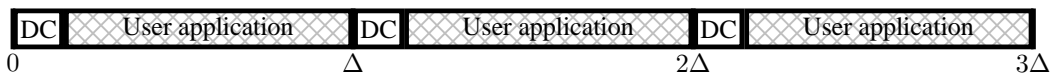
Figure 2: Division of time between the duty-cycling mechanism and user applications. The protocol works in a sequence of time periods of length \Delta . In each period, the first phase is dedicated to duty-cycling (DC), and the second phase to the user application.
