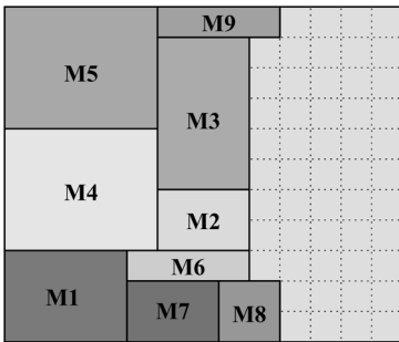
Fig. 10. Same FPGA as in Fig. 8 after successful defragmentation. The free space of 52 CLBs is the same as before. The largest free rectangle has grown to dimension 4 \times 11 and contains 44 CLBs. Now there are four free columns.
