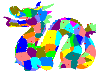
Figure 5: Voronoi diagram on the surface of the Stanford dragon; the data sites are marked as red points.
