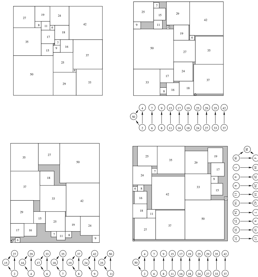
FIGURE 6.4. (a) An optimal packing of square21-0 of height 112; (b) an optimal packing of square21-mat of height 117; (c) an optimal packing of square21-tri of height 125; (d) a packing of square21-2mat of size 120x120.
