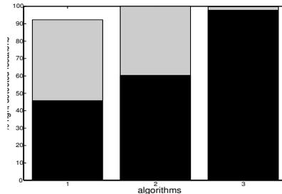
Fig. 4. Percent correctly detected semantic locations without (black) and with filtering on  $q > 0.8$  (grey) for (1) packet counting, (2) K Nearest Neighbors and (3) FIS
