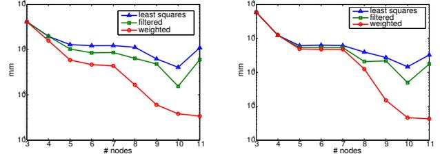
Fig. 9. Mean (left) and maximum (right) error of unweighted ( $\Delta$ ), weighted ( $+$ ) and filtered least squares multi-lateration algorithm
