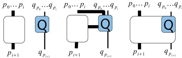
Fig. 8. Methods for integrating quality systems (Q) with a fusion algorithm: Independent(left), Filtering, Integrated (right)
