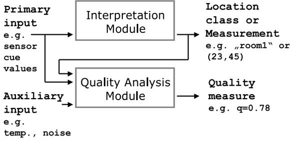
Fig. 2. Schematics of a general system for location measurement or classification with a parallel system for quality analysis.
