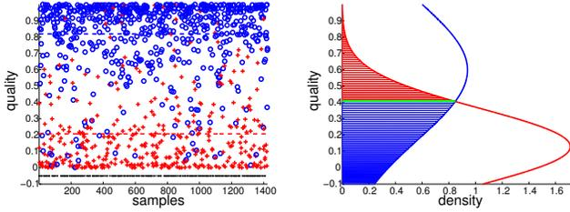
Fig. 6. Quality Measure (left, keys like Fig. 3) for test set 4; density functions (right) for accurate (top) and not accurate (bottom) measures; probabilities for false positives and negatives (shaded areas) regarding threshold  $\tau$  (green line)
