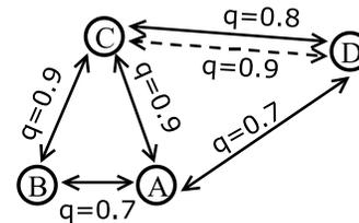
Fig. 1. Objects A-D in an environment with their quality based distance measurements
