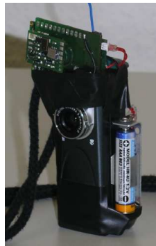
Fig. 10. Remembrance Camera (with Particle sensor node)
