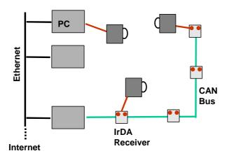
**Figure 2.** The network infrastructure of the Mediacup environment integrates IR, CAN, and LAN technoloogy.
