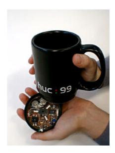
**Figure 1.** The Mediacup is an ordinary coffee cup with sensors, processing and communication embedded in the base.
