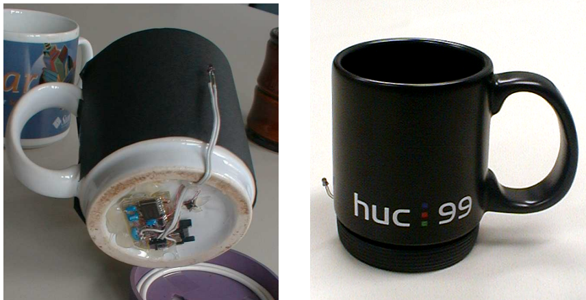
Fig. 5. MediaCup prototypes. Sensors, processor, and infrared diode are built into cup base.
