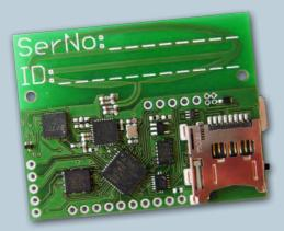
With 39 x 50 x 7 mm<sup>3</sup> INGA is relatively small and combines the advantages of other wireless sensor nodes. It is designed to be "lead-free" and for capacitors no "noble earths" (like tantalum) are needed. INGA consists of a two-layer PCB, with a printed antenna.
