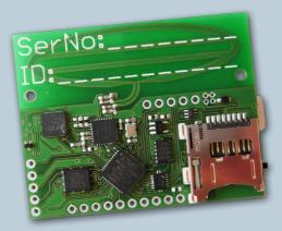
With  $39 \times 50 \times 7$  mm<sup>3</sup> INGA is relatively small and combines the advantages of other wireless sensor nodes. It is designed to be "lead-free" and for capacitors no "noble earths" (like tantalum) are needed. INGA consists of a two-layer PCB, with a printed antenna.
