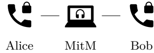
(a) Non-impersonating MitM: The attacker is a node in between and can forward as well as inject packets.
