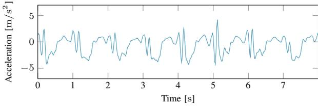
(a) Unmodified accelerometer reading (z-axis) at 50 Hz.
