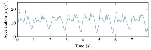
(b) After Madgwick's algorithm. Gravity  $g = \sim 9.81 \text{ m/s}^2$  can now be recognized, indicating a correct orientation relative to the ground.
