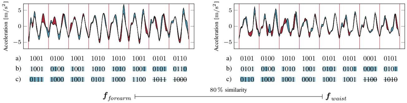
Fig. 4: Independent fingerprint generation on forearm and waist (forearm pre-processing is shown in Figure 2): Energy levels above the average gait cycle  $\mathbf{A}$  are blue and below red. After quantization in a), reliabilities are calculated and assigned to each bit in b). Darker color, indicates higher reliability. In c) the fingerprint is sorted by reliability vector of the forearm.
