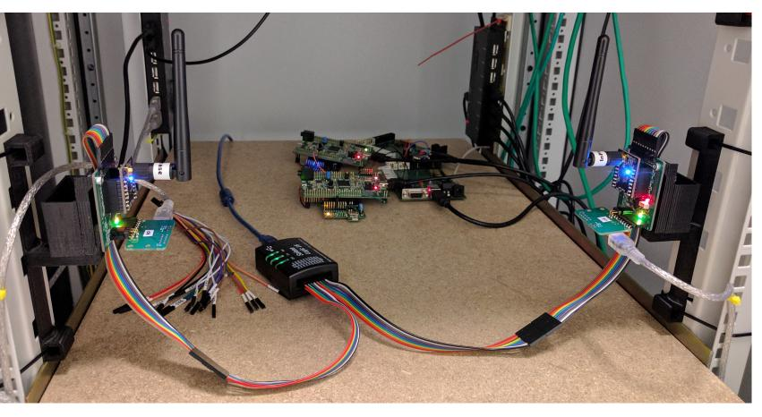
CI machine. A logic analyzer samples SPI and GPIO signals between radio and micro controller of both nodes. The data is automatically evaluated and a performance report is generated. It contains general fitness information of the ranging algorithm and regression test results. Raw data and the report are stored for later inspection.
