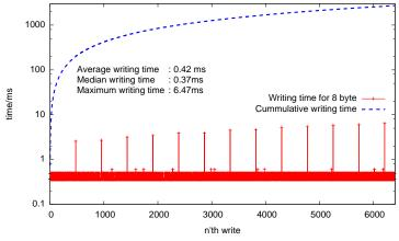
Higher delays, when needing to allocate a new RFS block
