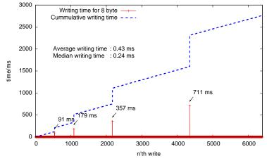
Write 6000  $\times$  8 bytes with a TMoteSky to a M25P80 flash memory
