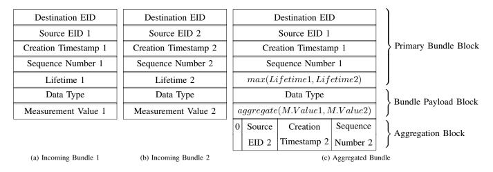
Figure 1: Bundle aggregation example with two (the same principle applies for more than two input bundles) incoming bundles and one outgoing bundle (shown bundles are simplified). Please note the matching *Destination EID* and *Data Type* fields.
