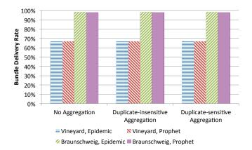
Figure 2: Bundle delivery rate for two routing protocols and two scenarios (higher is better).
