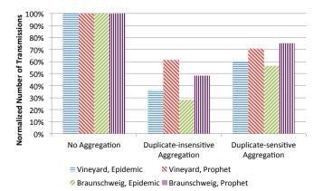
Figure 3: Total number of bundle transmissions for two routing protocols and two scenarios, normalized to "No Aggregation" (lower is better).
