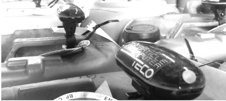
Fig. 1. Smart chemical drums equipped with sensor nodes
