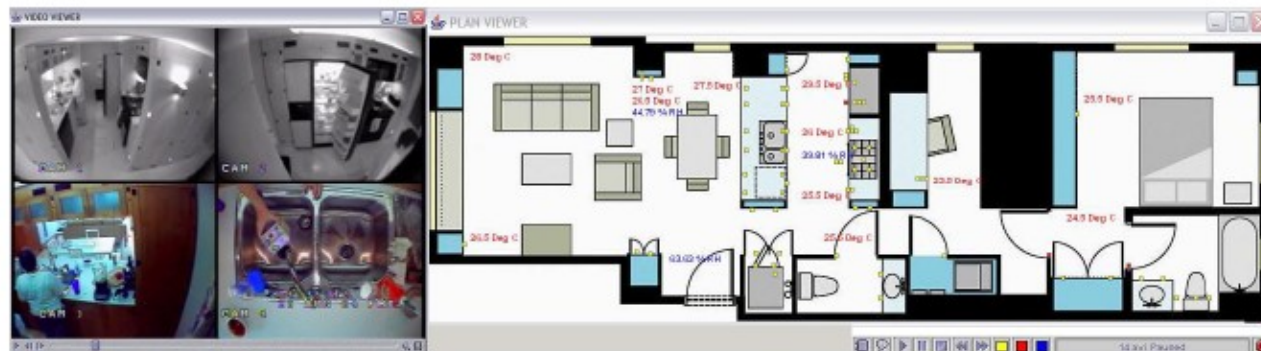
Figure 2: Annotation software permits the researcher to study data collected from the PlaceLab by watching 4 streams of automatically-selected “good” video views, listening to one automatically selected audio stream, and displaying sensor activations on a floor plan of the environment. Here the floor plan shows all switch sensors currently installed in the lab (small dots) and temperature sensor output. The researcher can use particular sensor activations to reduce the search and annotation time.
