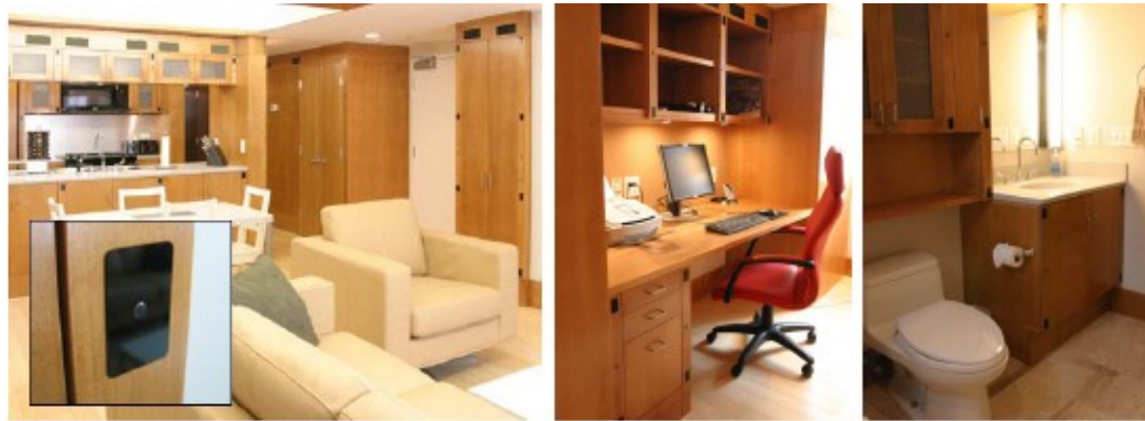
Figure 1: The PlaceLab living room and kitchen, office, and master bath. All of the observational sensing is built directly into the cabinetry. Although the sensors are ubiquitous, they become part of the design aesthetic (small black windows). Pilot volunteers have expressed that they are easy to forget. The inset in the left image shows a microphone.
