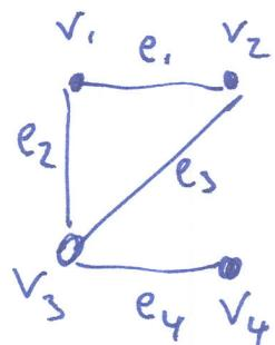
$$\begin{array}{c} v_1 \quad v_2 \quad v_3 \quad v_4 \\ \left( \begin{array}{cccc} 0 & 1 & 1 & 0 \\ 1 & 0 & 1 & 0 \\ 1 & 1 & 0 & 1 \\ 0 & 0 & 1 & 0 \end{array} \right) \end{array}$$
