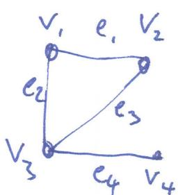
$$\begin{array}{c} e_1 \quad e_2 \quad e_3 \quad e_4 \\ \left( \begin{array}{cccc} 1 & 1 & 0 & 0 \\ 1 & 0 & 1 & 0 \\ 0 & 1 & 1 & 1 \\ 0 & 0 & 0 & 1 \end{array} \right) \end{array}$$
