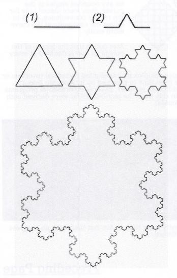
The genuine Von Koch curve, also called snowflake curve, is derived as the limit of a polygonal contour. At every step, as shown on the left, the middle third of every side of the polygone is replaced with two linear segments at angles 60° and 120°.
