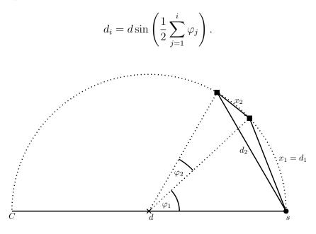
Figure 1: The first two steps of looking around a corner
