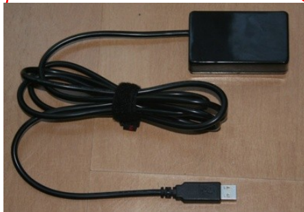
Sensor device for measuring the lever angle with an acceleration sensor
