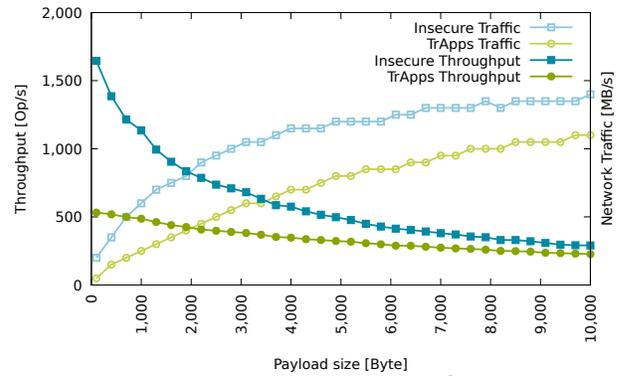
Figure 4: Throughput and network traffic of Secure Memcached.
