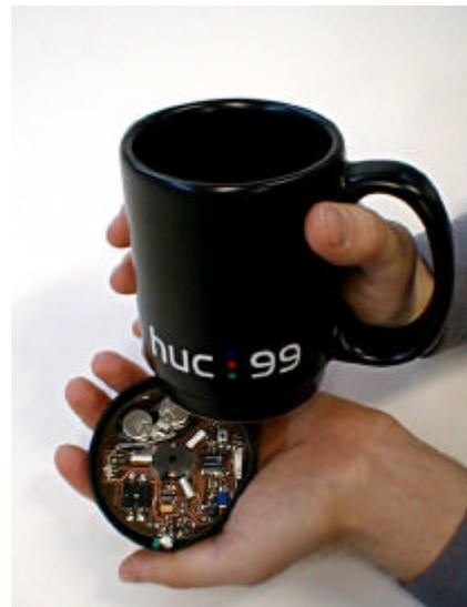
**Figure 1.** The Mediacup is an ordinary coffee cup with sensors, processing and communication embedded in the base.
