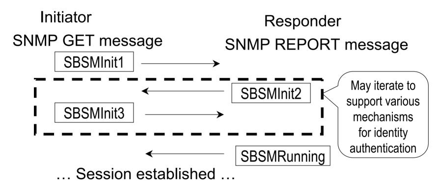
Note: for SNMPv3 messages containing SBSMInit[1,2,or 3] messages, the value for field *msgFlags* indicates *noAuthNoEncr* security level
