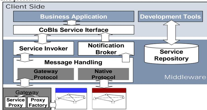
Fig. 3. CoBIs relocated process management architecture
