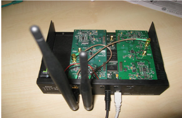
(a) A single USRP software radio with two transceiver boards
