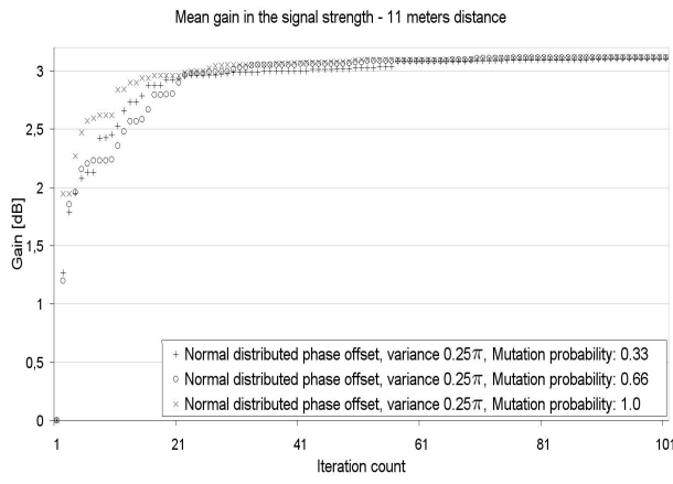
(c) Mean gain in the signal strength at a transmission-distance of 11 meters and a variance of the random process of 0.25\pi for 100 iterations
