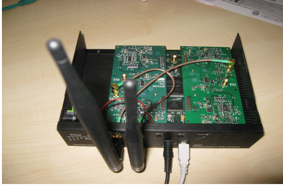
(a) A single USRP software radio with two transceiver boards
